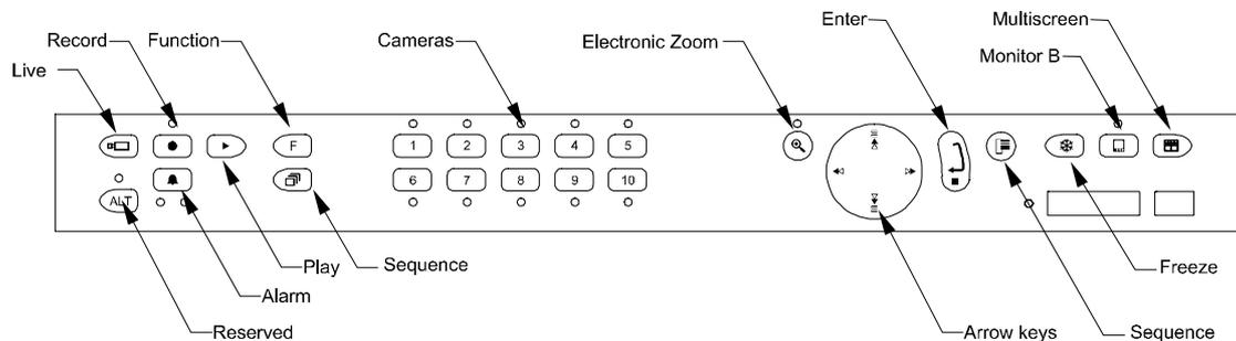
Figure 3 ZMX/CS/10 Front Panel
