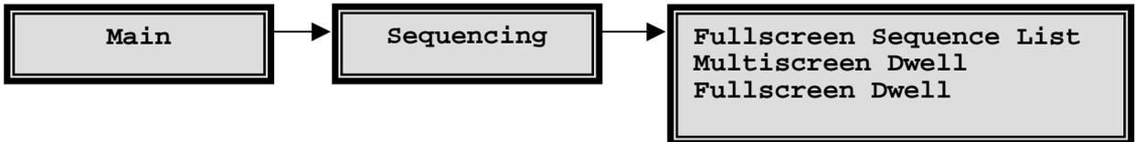
There is one full-screen sequence list which operates on both Monitor-A and Monitor-B. The list has 30 entries.
