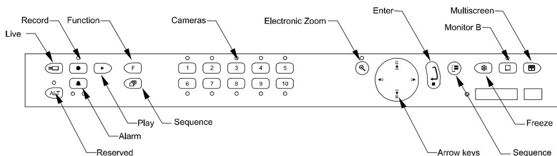
Figure 1 The multiplexer Front Panel
