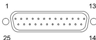
Figure 5 The 25-way D-type Connector Numbering
