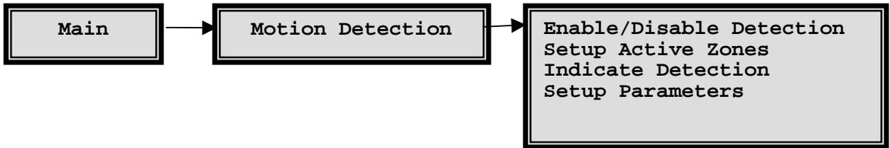
The multiplexer offers comprehensive motion detection capabilities, including sensitivity settings and detection area selection per camera. Motion detection is used to adjust the rate at which cameras are recorded.
