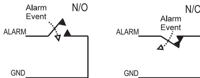
Figure 6 Normally-Open and Normally-Closed Connections
