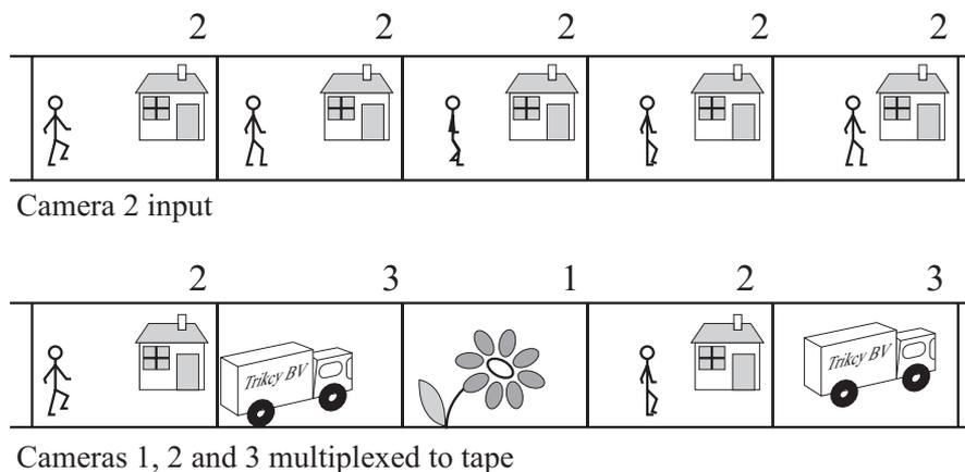
**Figure 2 Illustration of Multiplexing**
