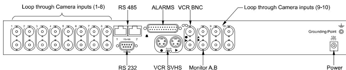
**Figure 2 Multiplexer Back-Panel Connections**
