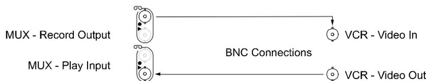
**Figure 4 Standard (BNC) VCR connections**
