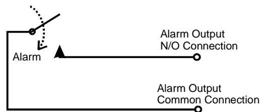
Figure 7 Alarm-Output Relays, Internal Circuitry
