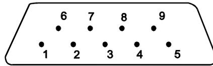
Figure 9 9-way Connector Numbering
