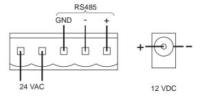
IMPORTANT: The 24 VAC power supply must be a class 2 type. Do not make any connection to ground.
